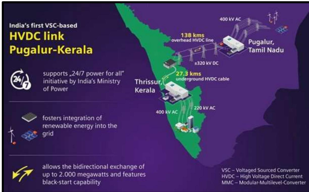
POWERGRID has totally commissioned India's 1st Voltage source converter (VSC) based mostly High Voltage direct current (HVDC) System.
